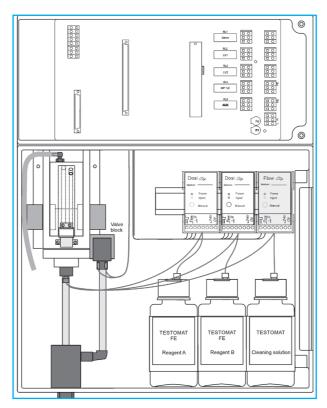
Internal design with three dosing pumps for precise analysis of iron content and cleaning function for flushing the measuring chamber.
